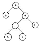
The initial call to **GenerateCode** is with a pointer to the '+' and result register 0.
